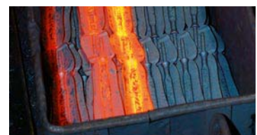
Freshly forged and still glowing red, the blanks wait for the next process.
